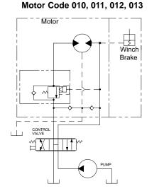
The friction brake is a load holding brake only and has nothing to do with dynamic braking or rate of descent of a load.
