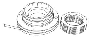
New lobed steel brake separator plates and motor support. Note groove on outside diameter of motor support.
