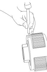
1. Remove the planet gears by driving the roll pins into the center of the planet shafts.
