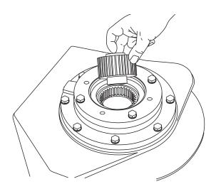
12. Install the brake clutch assembly.
