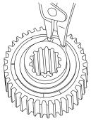
4. Remove the snap ring and sprag bushing retainer from one end only of the brake clutch assembly.
