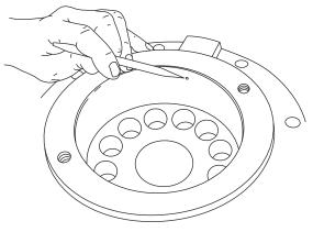
1. Thoroughly clean and inspect all parts at this time. Check brake piston sealing surfaces on brake cylinder and motor support for scoring or wear. Be sure brake release port is free of contamination.
