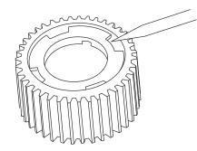
Press a sprag bushing into the outer race, using a mechanical or hydraulic press. A flat plate of approximately the same diameter as the bushing flange outside diameter should be placed between the press and bushing during assembly to protect the bushing. Be certain the bushing flange is against the shoulder in the outer race.
