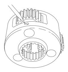
4. Note that the roll pin is slightly recessed in the carrier when properly installed. With a center punch, stake the carrier next to the pin hole as shown. This will distort the hole so the pin will not back out. Repeat these steps for each of the three planet gears.
