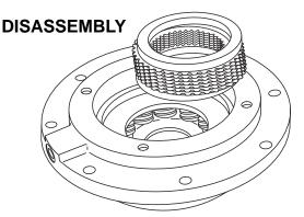
1. After removing the motor support and brake clutch assembly, continue brake cylinder disassembly by removing the spacers, friction brake discs and steel brake discs.
