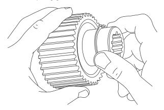
5. Slide the inner race through the bushings and sprag clutch (the race will have to be rotated in the free-wheeling direction to start it through the sprag clutch). If the inner race will not go through the bushings, the bushings have probably been damaged and should be replaced.
