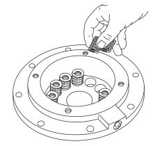
3. Remove the brake springs.
