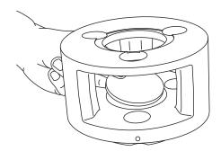
1. Place the output planet carrier on workbench with splined coupling side down. Install output thrust plate in center of carrier.
