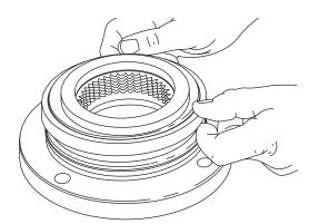
Lubricate the brake piston seal and motor support sealing surface with petroleum jelly or hydraulic oil. Install new piston seal to motor support, seal lip down.
