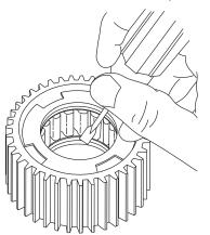
Use a screwdriver and mallet to remove the sprag bushing from one end of the outer race. There are four special cut-outs in the bushing for this purpose. Be careful not to damage the bushing inside surface. If a bushing's inside surface is damaged or shows wear, replace it.
