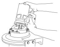
2. Stand the hoist on the bearing support plate. Remove the brake release tube assembly (59) between the brake valve block and the brake cylinder end plate. Remove the capscrews and lockwashers which secure the motor to the motor adapter, and lift the motor out of the motor adapter. Remove and discard the O-ring installed on the pilot of the motor.
