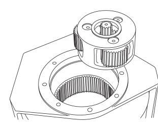
5. Stand hoist on bearing support end. Install the output sun gear and thrust washer into output planet carrier.
