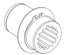
4. Next, install a sprag bushing retainer, then a snap ring on the inner race. Be sure the snap ring is seated in the snap ring groove.
