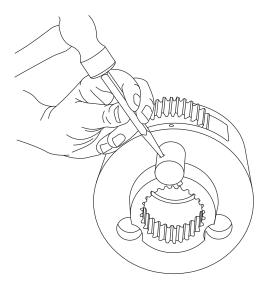
2. Use a punch to drive the roll pins from the planet shafts. Do not reuse the roll pins.
