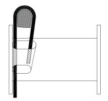
The standard cable anchor wedge supplied with the hoist is intended for 5/16 to  $\frac{1}{2}$  in. (8 to 13 mm) wire rope.
