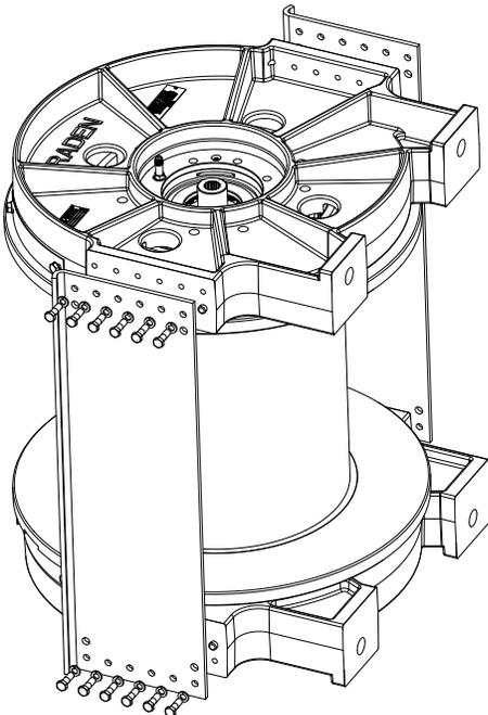
3. Remove the 24 capscrews and lockwashers securing the tie plates (Item 1) to both end brackets and remove the tie plates. The tie plates have two dowel pins in each end and may have to be lightly tapped or pried
