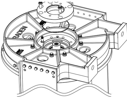
2. Remove the four capscrews from the motor adapter and remove the motor adapter on SAE C motor only (Item 40) from the drive gearbox. Remove and discard the O-ring (Item 38) from the motor adapter.
