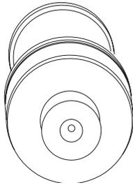
2. Inspect the 0.020-inch (0.5 mm) orifice in the end of the spool to be certain it is open. On the 1-1/4-inch valve, also inspect the pilot orifice to be certain it is open.
