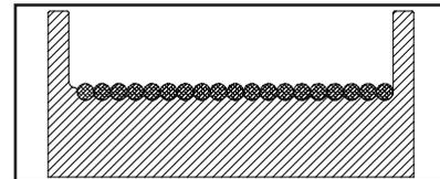
**NOTE:** Only one size cable can be used on a grooved drum.
