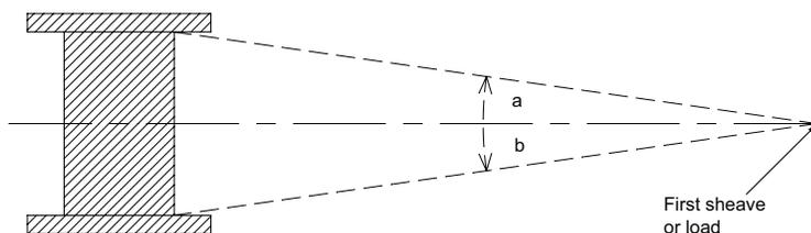
First sheave or load should be centered between the drum flanges, so that angle A and angle B are equal.
