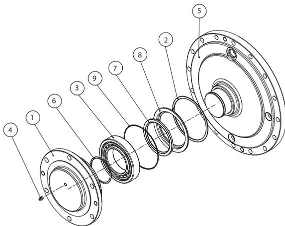
6. Secure outer hub with bearing and seal container in place on the hoist side plate using lockwashers (10) and capscrews (9). The outer hub should be positioned so that the grease fitting is at the 12 o'clock position with the hoist mounting feet setting on the ground. Torque capscrew (9) to the torque chart value given in this manual for 5/8-inch bolts.
