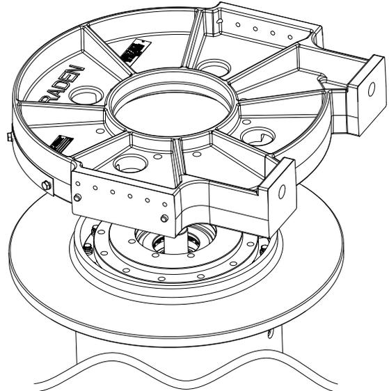
5. Lift the motor end bracket (Item 25) from the drum/drive assembly.
