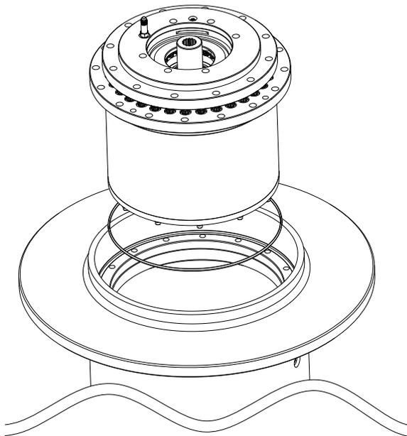
7. Lift the hoist drive gearbox out of the drum using two 3/4 NC eyebolts spaced 180 degrees apart as lifting lugs. Refer to Hoist Drive/Gearbox Service section for further disassembly of hoist drive
