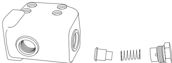
4. Remove the check valve spring retainer, spring and check valve poppet.
