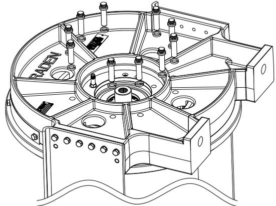
4. Remove the ten 12 pt. capscrews (Item 23) and lockwashers (Item 24) securing the end bracket (Item 19) to the gearbox. Use overhead hoist/chain to support end bracket/drum during tie plate removal.
