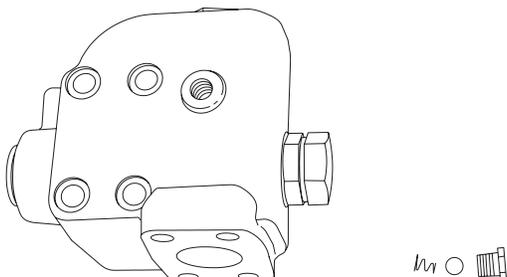
2. Remove the fitting, motor drain check ball and spring.
