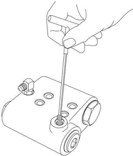
1. On the 1-1/4-inch valve only, remove pilot orifice from the brake release port using a 5/32-inch Allen wrench.
