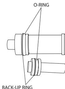
2. Install new O-rings and backup rings on the spool and damper pistons as shown. It is important that each backup ring is on the correct side of its O-ring. Take care not to cut the O-rings during assembly. Let the spool and piston set for ten minutes before installing them in their respective bores. This will allow the O-rings to return to their original size after being stretched.
