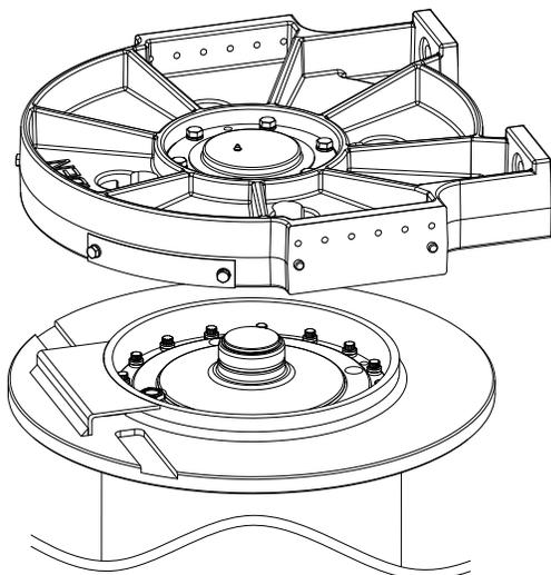
1. Lift the support end bracket from the drum.
