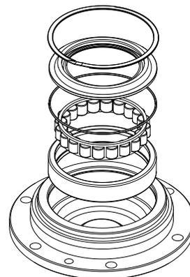
2. The outer hub (Item 1) is in the end bracket, and the drum support (Item 3) is in the drum. Remove the retaining ring (Item 2) and the seal carrier and seal (Items 6 and 7). Remove and discard O-ring (Item 9). Remove the seal from the seal carrier and discard.
