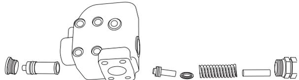
3. Remove the spool spring retainer and spool spring. Remove the spool plug and carefully remove the spool assembly. Remove the damper piston from the spool. The piston will come out of the spool slowly, because of a partial vacuum formed between the two. Use extreme care to avoid damaging the polished surfaces of either piece.
