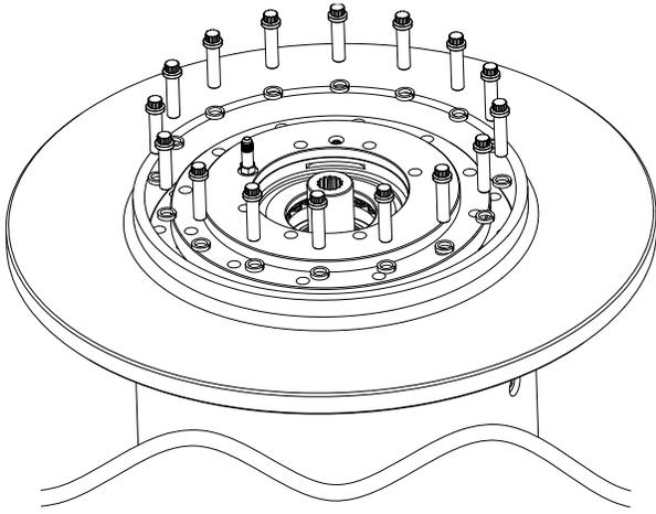
6. Remove the hex-head capscrews and lockwashers (Items 30 and 22) that secure the gearbox to the hoist drum.
