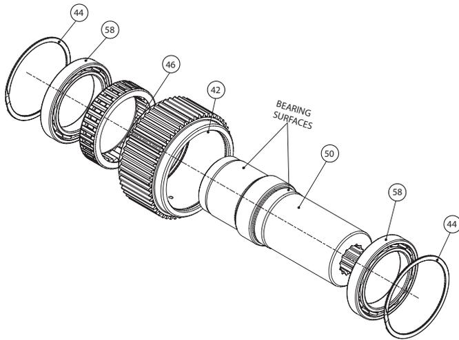
**NOTE:** Outer race (Item 42), Inner race (Item 50) and overrunning clutch (Item 46) are NOT SOLD individually as replacement parts. If any of these parts require replacement, the entire overrunning clutch assembly must be replaced. Carefully note the relative orientation between the inner and outer races, and the direction of free rotation of the inner race. The clutch MUST be re-assembled correctly for proper hoist operation.
