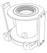
7. Lubricate the bearing support and sealing surface with petroleum jelly or gear oil and place the cable drum (3) on the bearing support endplate. Check that the drum rotates freely on the bearing.
