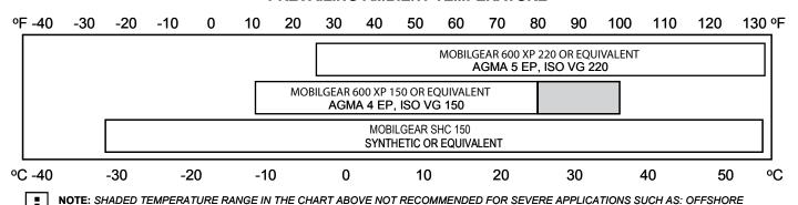
Planetary hoists are factory filled with Mobilgear 600 XP 150, or equivalent. Consult your oil supplier for other equivalent oils if required.
