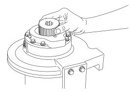
3. Remove the brake coupling (29) and sun gear (41) from the hoist.
