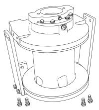
4. Remove the four capscrews (5) and lockwashers (6) holding the tieplates (4) to the brake cylinder endplate. The drum is supported on the endplate by a large bushing. Carefully separate the endplate assembly from the drum. The endplate assembly includes the static brake cylinder. Remove the brake cylinder endplate from the drum.
