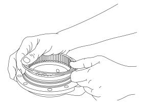
1. Place the motor adapter on workbench with the motor mounting surface down. Install a new O-ring (36). Lubricate the brake piston seal with petroleum jelly or hydraulic oil and install on the motor support with the seal lip down, as shown above.
