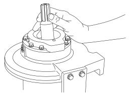
10. Fasten the two tie plates to the endplate with capscrews (5) and lockwashers (6), and torque all eight (8) tie plate capscrews to their proper value. Check that the drum turns freely in both directions without binding or any interference. Install the sun gear (41), meshing with the teeth on the planet gears in the drum.
