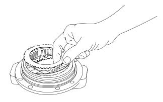
2. BG4B (current) units with "lobed" brake discs: Install a steel brake disc (35) into the motor support, followed by a friction disc (34). Alternately install steel and friction discs until eight (8) friction and nine (9) steel discs have been installed. Finish with a steel disc on top.
