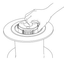
8. Install the planet carrier assembly into the drum while meshing the planet gears with ring gear and the planet carrier with the bearing support.
