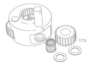
1. First drive the rollpins (17) into the center of the planet shafts (14). Now you can remove the planet shaft (14), two thrust races (16), planet gear (13) and roller bearing (15). Repeat this procedure for the other two planet gears. Thoroughly clean all parts and inspect for damage and wear. The bearing rollers should not exhibit any irregularities. If the rollers show any sign of spalling, corrosion, discoloration, material displacement or abnormal wear, the bearing should be replaced.
