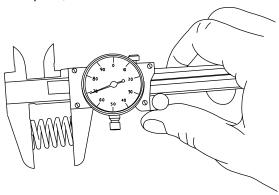
4. Check free length of each brake spring. Minimum free length is 15/16 inch (23.8 mm). Check springs for any signs of cracking or failure. If a brake spring must be replaced for any reason, then **ALL** brake springs must be replaced.
