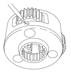
3. With a center punch, stake the carrier next to the pin hole as shown. This will distort the hole so the pin will not back out when in service. Repeat these steps for each of the three planet gears.
