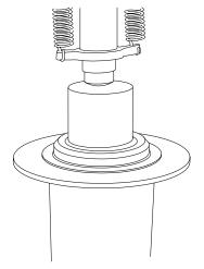
2. Install new bearings in the drum if replacement is necessary. Apply a non-hardening sealant on the outside diameter of each new seal and press the seals into the drum, using a flat plate to avoid distortion.
