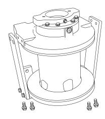
9. Lubricate the bearing support and sealing surface on the brake cylinder endplate and install the endplate assembly onto the drum.
