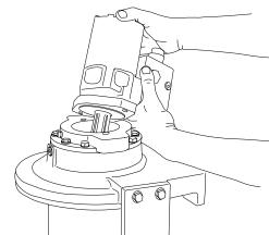
12. Install a new gasket (37) on the motor pilot and lubricate with petroleum jelly or gear oil. Install the motor onto the motor adapter with two (2) capscrews (50) and lockwashers (51). Torque the capscrews to their proper value.
