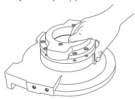
5. While holding the motor adapter and brake assembly together, turn it over and install into the brake cylinder endplate. Install the eight (8) capscrews (47) and lockwashers (48) but do not tighten them completely at the same time.
