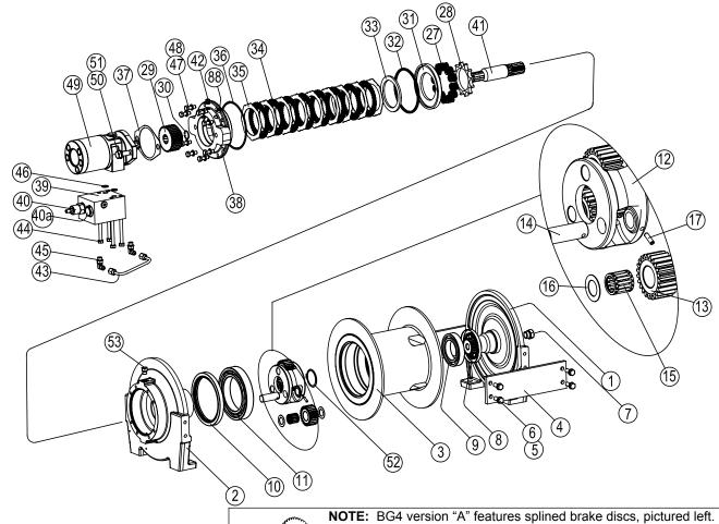
**NOTE:** BG4 version "A" features splined brake discs, pictured left. The "B" version features lobed discs as shown in explosion above. Additionally spring count and brake disc count (items 27, 34, & 36) may vary from depiction above; consult the appropriate Material List for your particualr hoist model for accurate brake spring and brake disc quantities.
