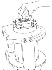
11. Install the brake coupling into the brake pack with the flat end of the coupling toward the motor. Turn the coupling back and forth to align the outer splines with the brake disc splines. The coupling must engage all the brake discs and the snap ring in its center must rest on the sun gear. Evenly tighten the eight (8) capscrews around the motor adapter one turn at a time until the motor adapter is firmly seated to the endplate. Torque the capscrews to their proper value.
