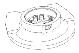
4. Install the spring locator (28) and the eight (8) springs (27) into the brake cylinder end plate (2).
