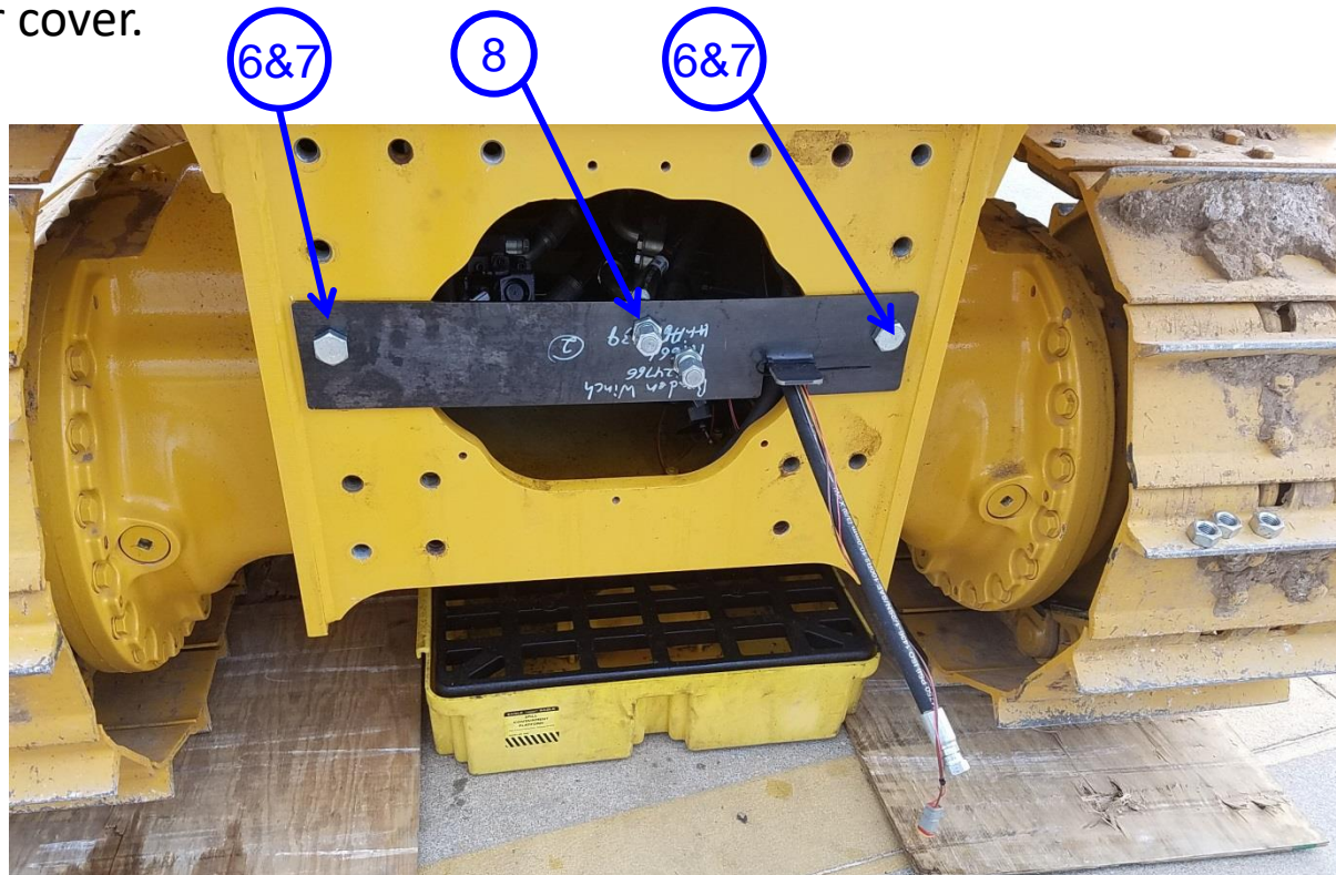
Fig. 10 – Center cover installation. 68069_A_B120 LIT2797
