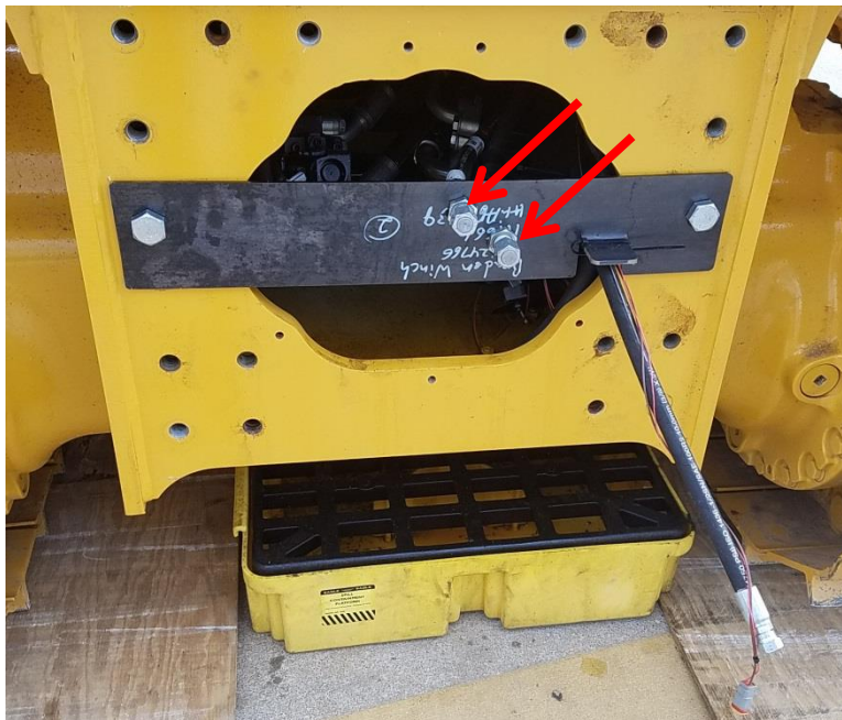
INSTALL EXISTING TRACTOR HOSES & BULKHEAD FITTINGS
